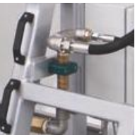
Automated test sample supply directly from the cooling chamber (Model 1671)
