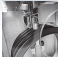
Automated measurement and storage of the dropping speed at impact
