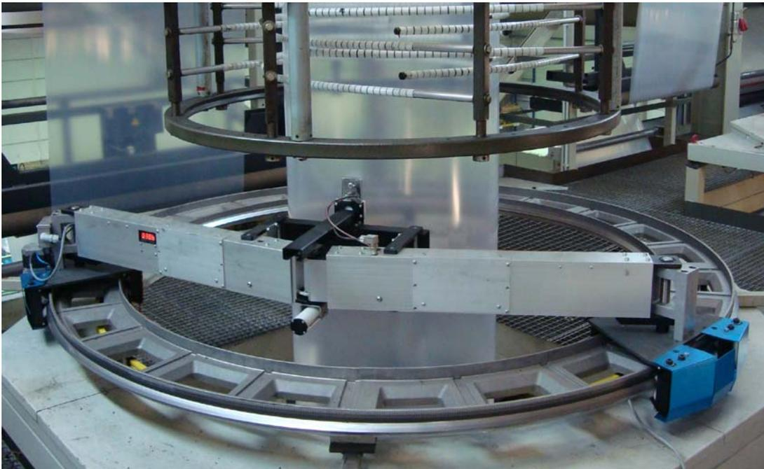
Several thickness sensors with different coatings can be used with the K-300 measuring electronic box. A quick disconnect allows to change the sensor in seconds.
