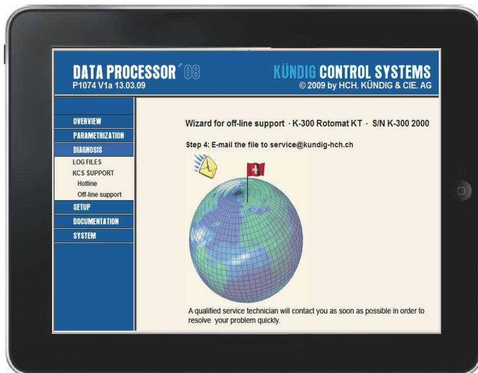
The data processor comes with a user friendly web interface, which allows output of process data and thickness profiles, as well as system configuration and troubleshooting. Remote access to the data processor through the internet is also available.
