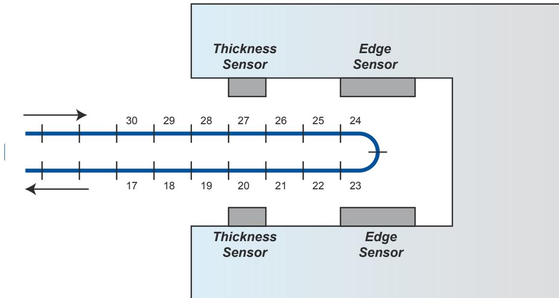
The complete film perimeter will be divided in several sections. The thickness sensor measures the sum of the upper and lower film sections. The rotating movement of the haul-off or the die causes a continuous variation of the measured sections.
